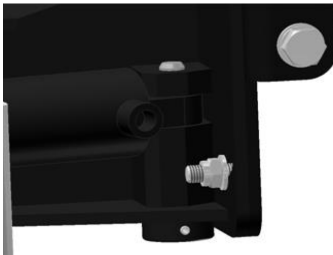
Fig 16: Attachment points of the swing cylinders
