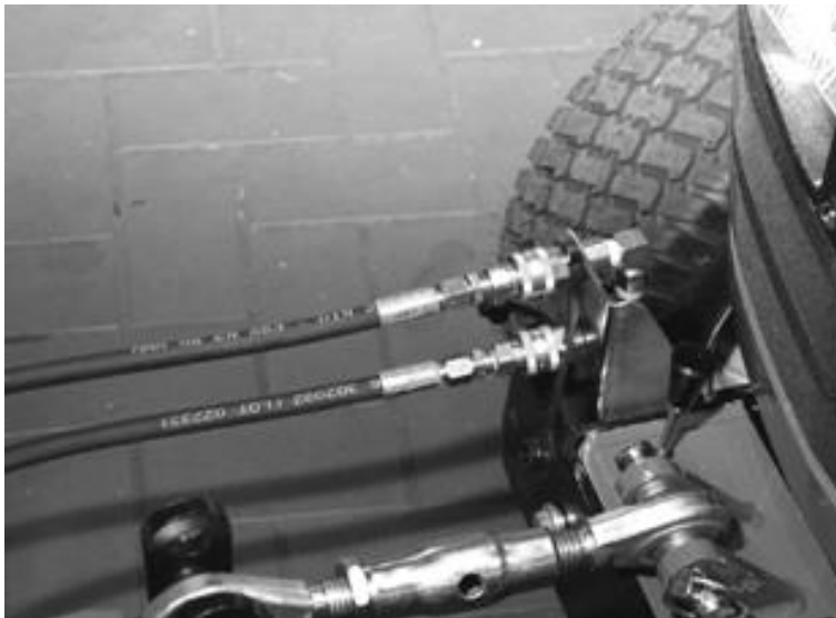
Fig. 9: Connecting the hydraulic lines on the tractor hydraulic system
