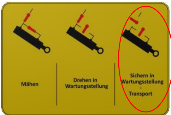
Fig. 36: The shut-off valves "Secure in maintenance position"
