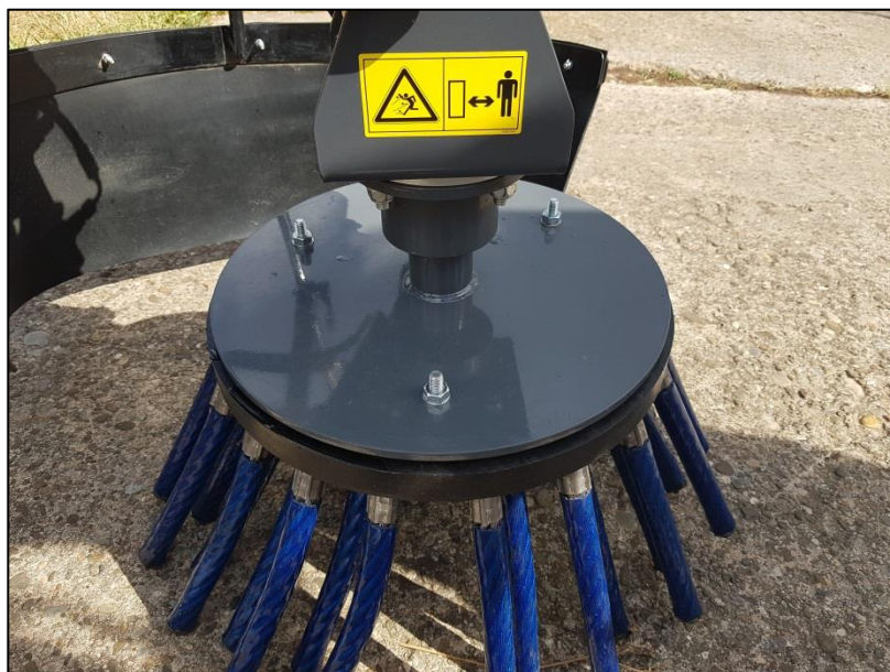
Fig. 26: Replacing the brush
