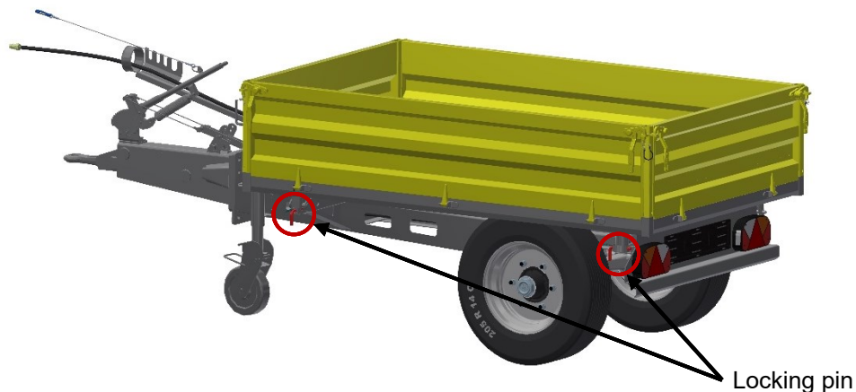
Fig. 21: Load bed locking mechanism
