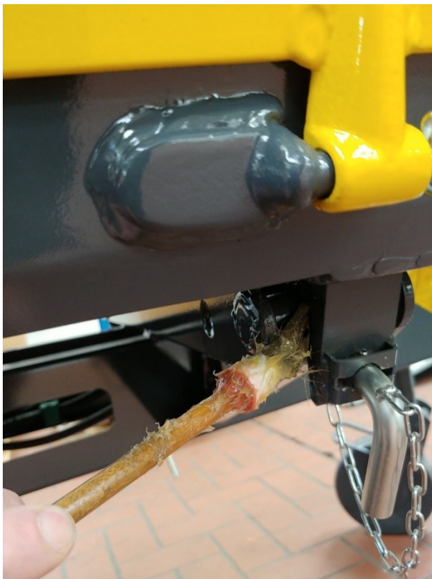
Fig. 25: Lubricate the dumping mechanism
