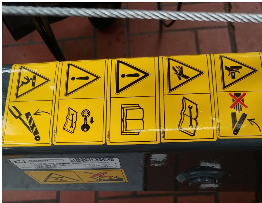
Fig. 6: Safety stickers on the drawbar
