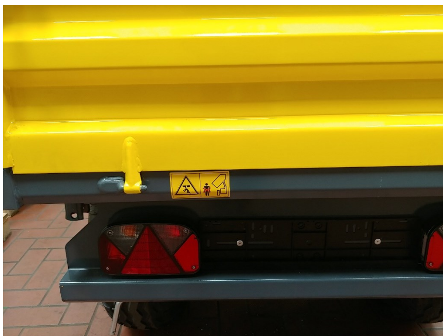
Fig. 10: Safety stickers trailer rear
