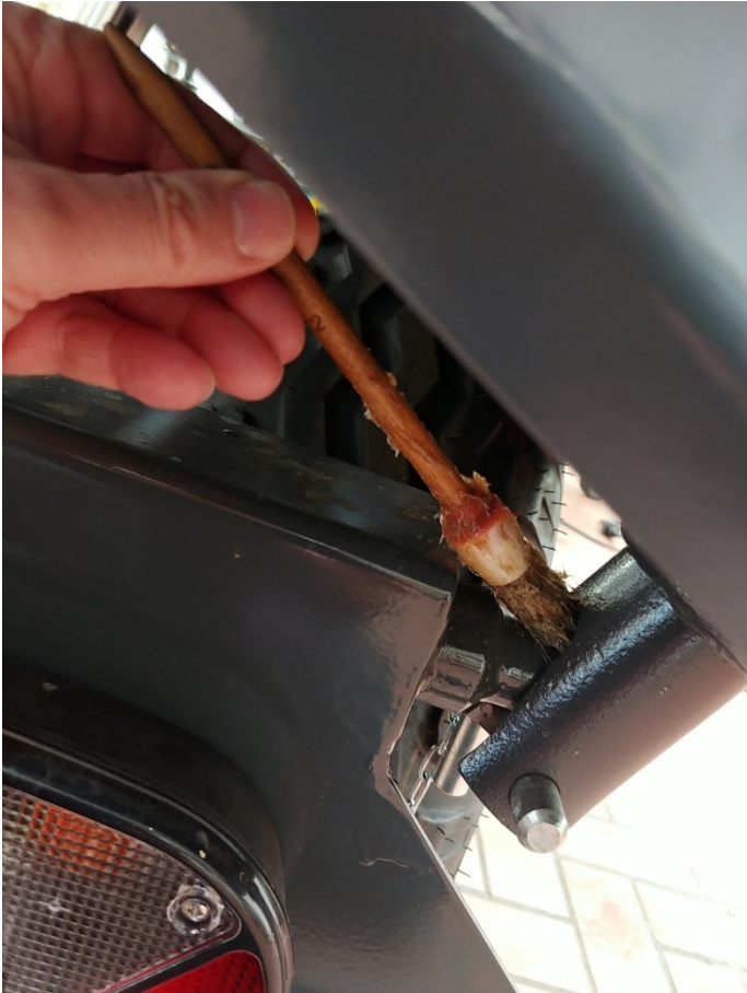
Fig. 26: Lubricate the dumping mechanism
