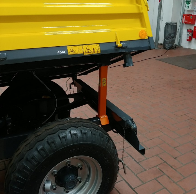
Fig. 12: Safety stickers lowering safeguard
