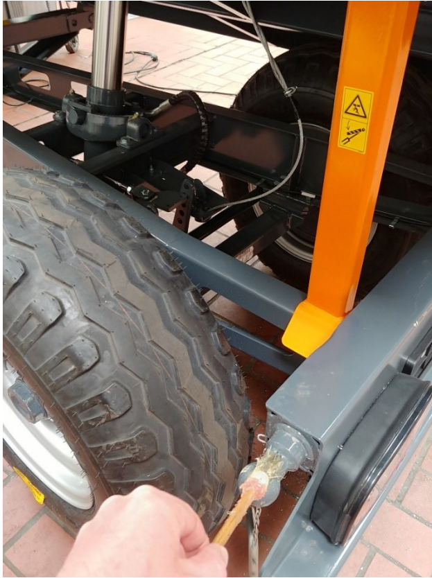
Fig. 24: Lubricate the dumping mechanism
