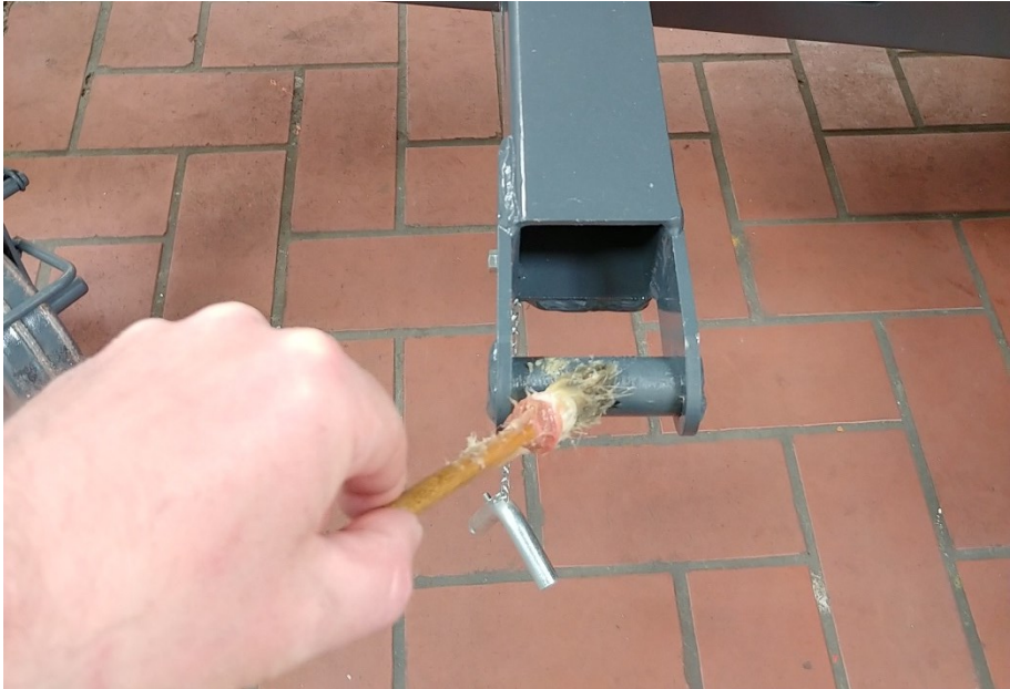
Fig. 23: Lubricate the dumping mechanism
