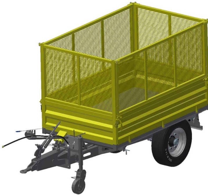
Fig. 18: Grating height extension
