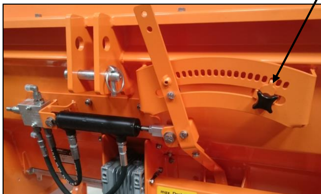
Fig. 9: Hydraulic dosing flap actuation
