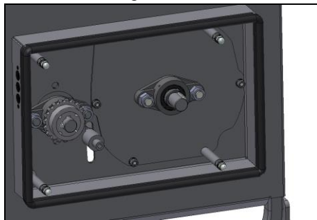
Fig. 30: Opening the chain housing
