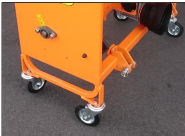
Fig. 17: Wheel set mounted on spreader
