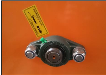
Fig. 24: Pedestal bearing on left in direction of travel
