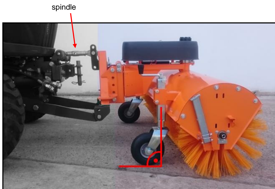
Figure 32: Adjust the inclination of the sweeper
