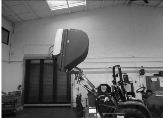
Fig. 9: Container lifted out, cover closed.
